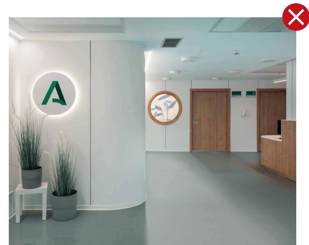
Potentially confusing reflections and glare
